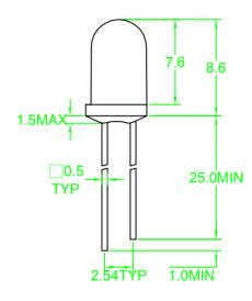
NOTE:1.All dimension are In millimeters tolerance Is  $\pm 0.25$  unless otherwise noted 2.Specifications are subject to change without notice
